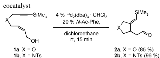
Scheme 1. Pd-Catalyzed Cycloisomerization of Yne Allyl alcohols 1 with 20 % N -Acetyl Phenylalanine as Acid Cocatalyst
